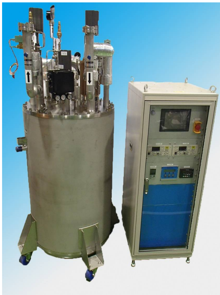
The LN 2 circulation cooling system proposed by SSK.
